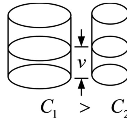
$$q_1 = C_1 v \quad > \quad q_2 = C_2 v$$
